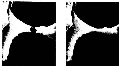
Figure 8. Blown and Unblown Polysilicon Fuse.
